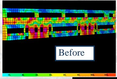
Reduces stress in walls, and reduces load in concrete frame
