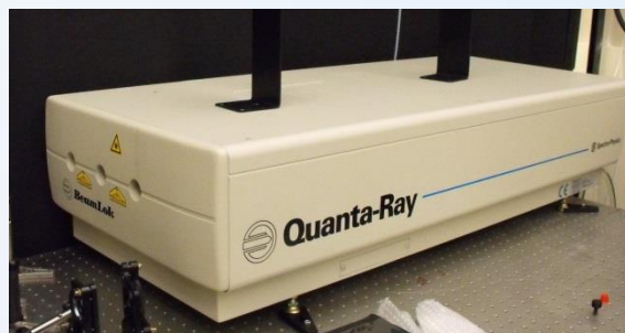
Spectra Physics 50Hz Laser
