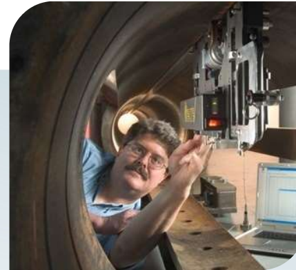
Robotic Instrument for Catapult Inspection
