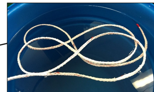
Photodetecting fiber woven into rope engineered for positive buoyancy (MicroAward w/ Teufelberger)
