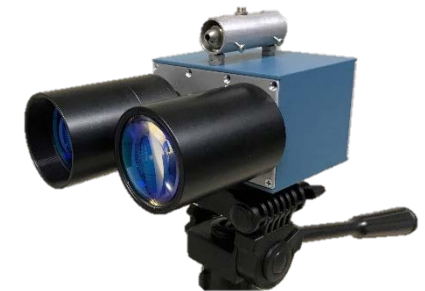
Designed & built an optical Tx/Rx module for testing and evaluation of IFF & voice comms
