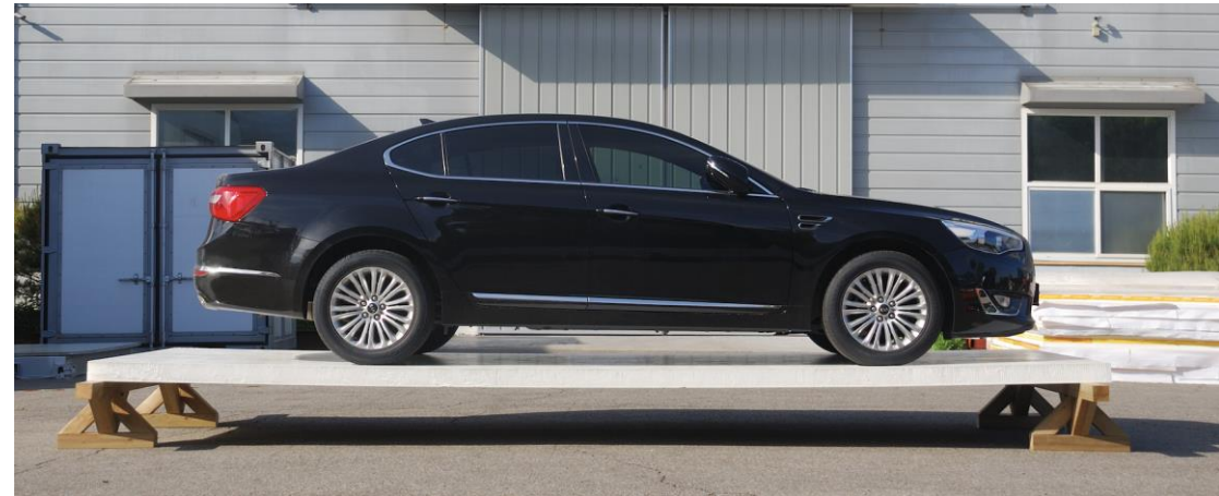
4" thick composite panel (composite skin thickness 0.03", FR EPS 1.89")
