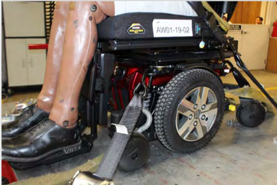
Front tie-downs in simulated taxiing setting
