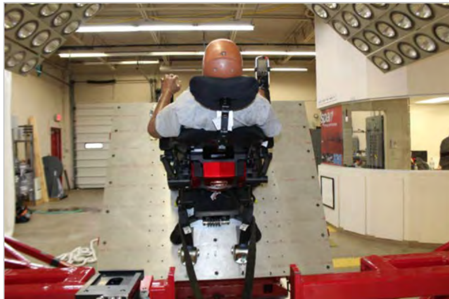
Rear tie-downs in a simulated crash setting
