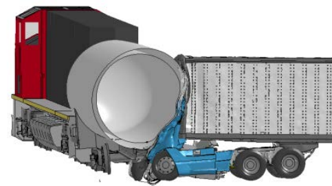
Figure 49. Tractor-trailer impact response on the tender.
