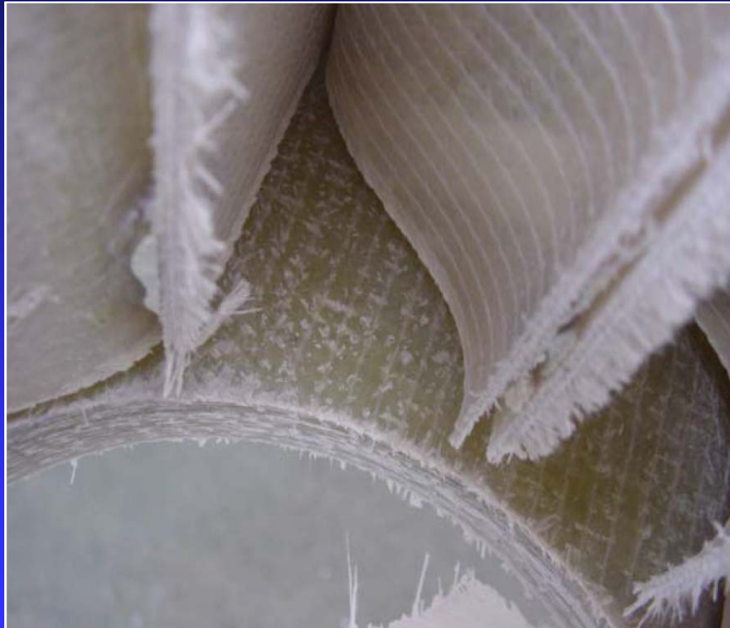
Figure 9-8. No Adhesive Between Facesheet and Core Webs.
