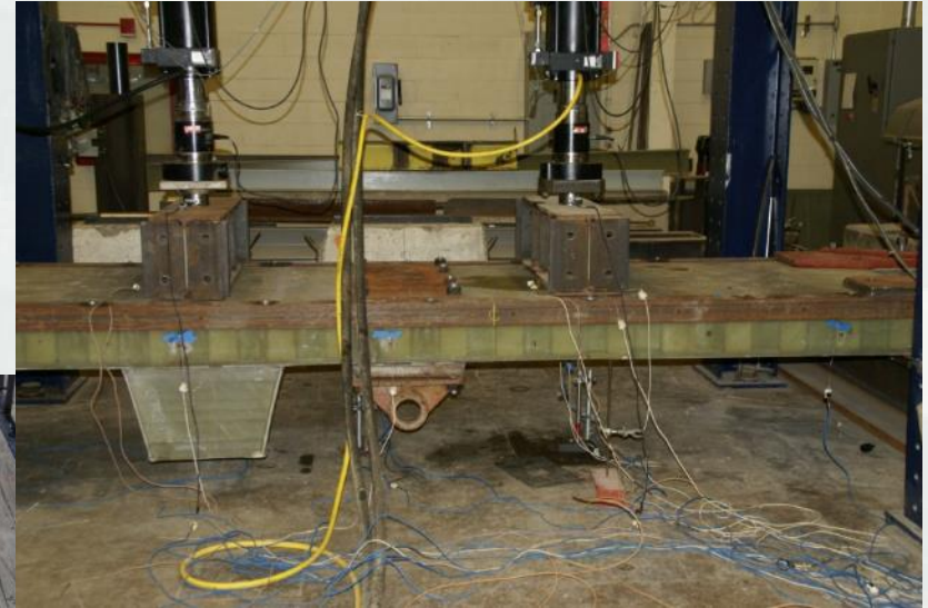
Tested to twice the working load of a timber wicket.
