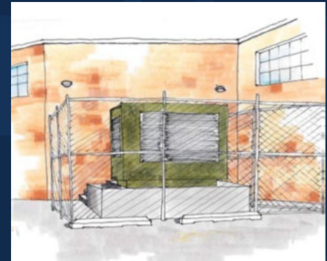
Elevate electrical systems
