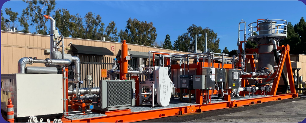
Fluidized Bed Connected to a Diesel Generator
