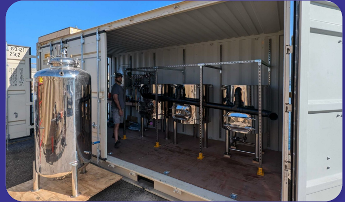
Separate Adsorber and Packed Columns
