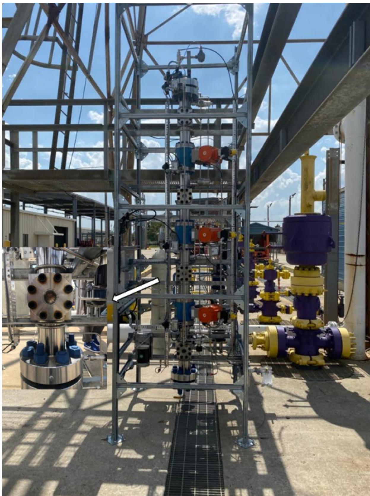
Figure 4: High Pressure Riser - Gas Mass Transfer Apparatus developed and commissioned under this project.
