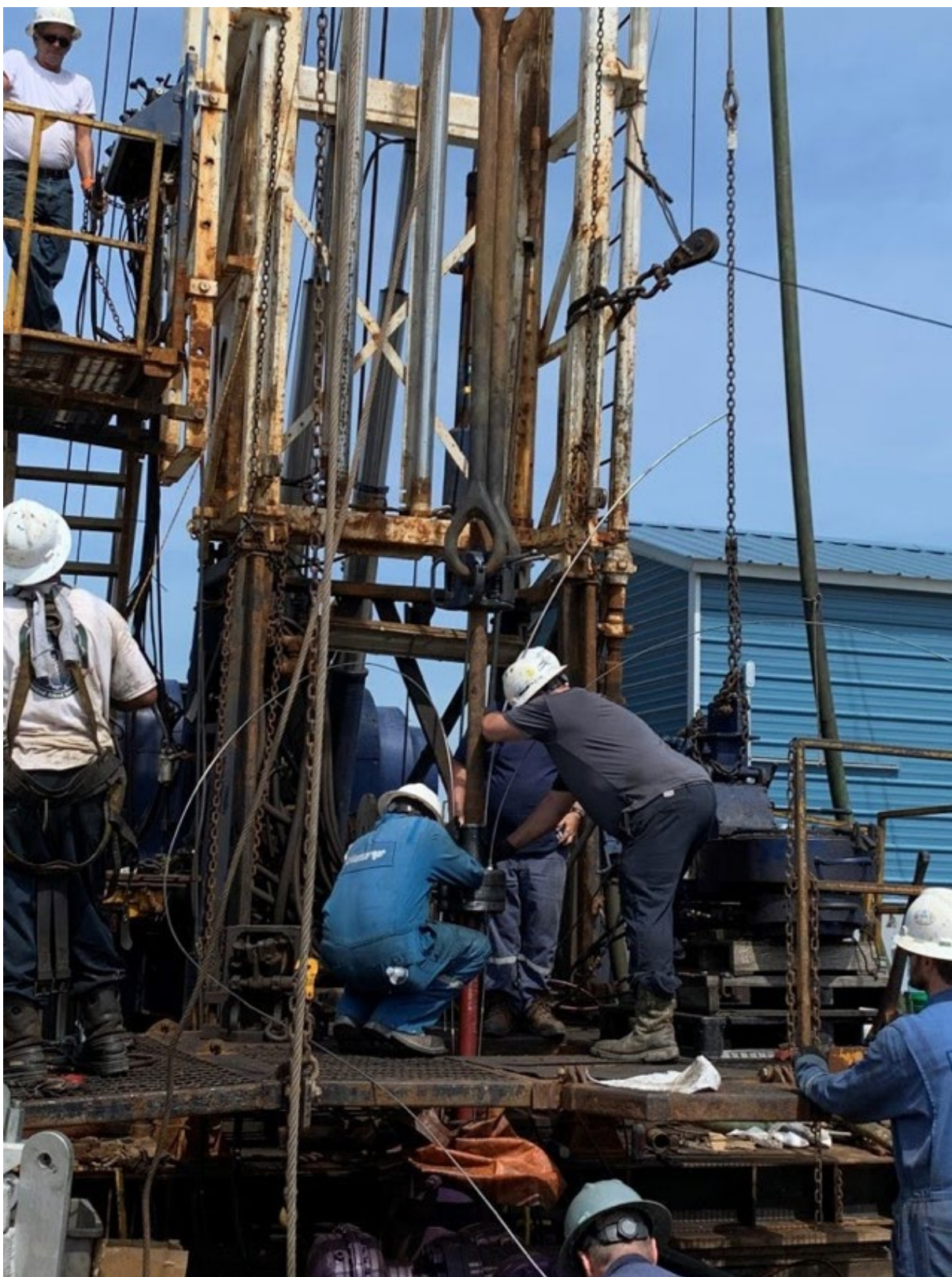
Figure 3: Workover done on Well No.2 to install Distributed Acoustic Sensor, Distributed Temperature Sensor and downhole pressure-temperature gauges.
