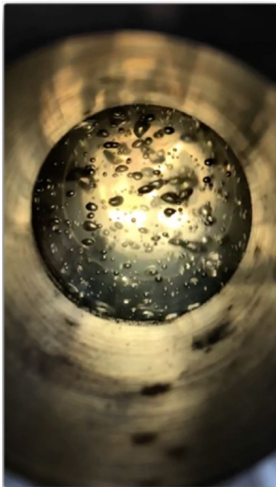
Figure 7: A snapshot of a video recorded through the sapphire observation window on the outdoor high-pressure mass transfer apparatus for the assessment of gas velocity and bubble size distribution.
