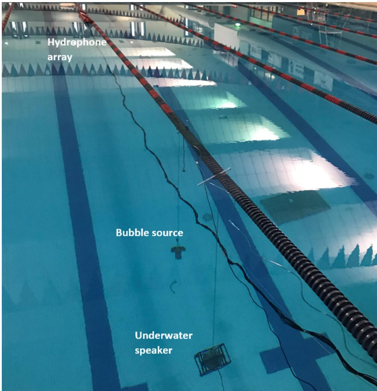
Figure 3-5: Swimming pool test.
