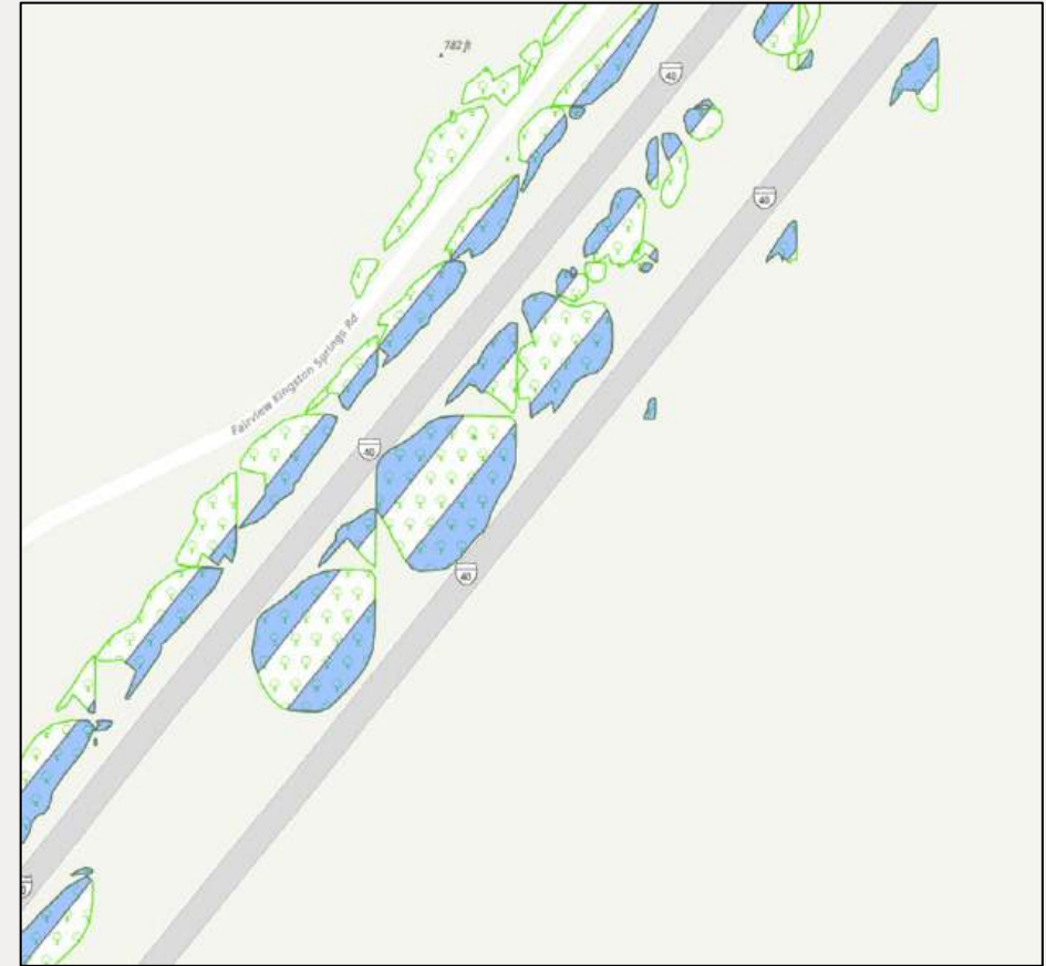
TRAM map showing the locations of trees (green) along an interstate route that require removal (blue) based on street-level, high-resolution imagery
