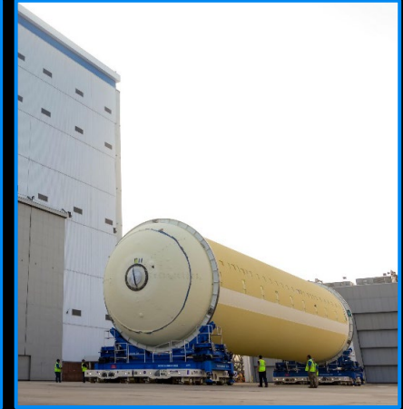
Thermal protection system applied to the SLS liquid hydrogen tank: May 14, 2025
