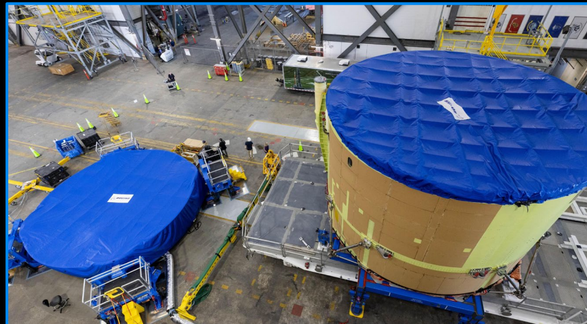
First pieces of flight hardware for Artemis III, the SLS rocket's boattail and engine section, arrive at Kennedy's VAB: July 30, 2025
