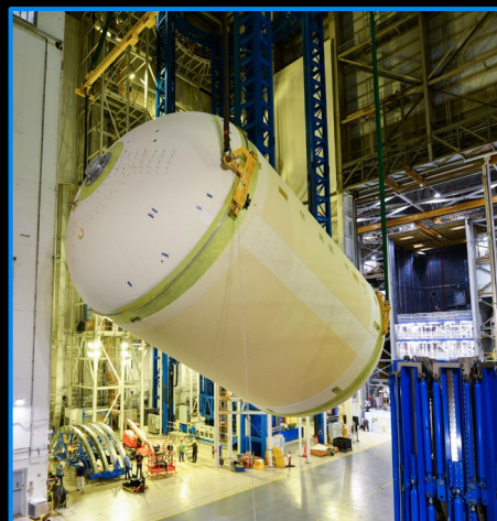
Core stage liquid oxygen tank lifted into vertical position at NASA Michoud: July 18, 2025
