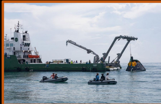
More recently, teams from NASA and DOD rehearsed abort scenario recovery procedures with the Crew Module Test Article. [VALENT] June 12, 2025
