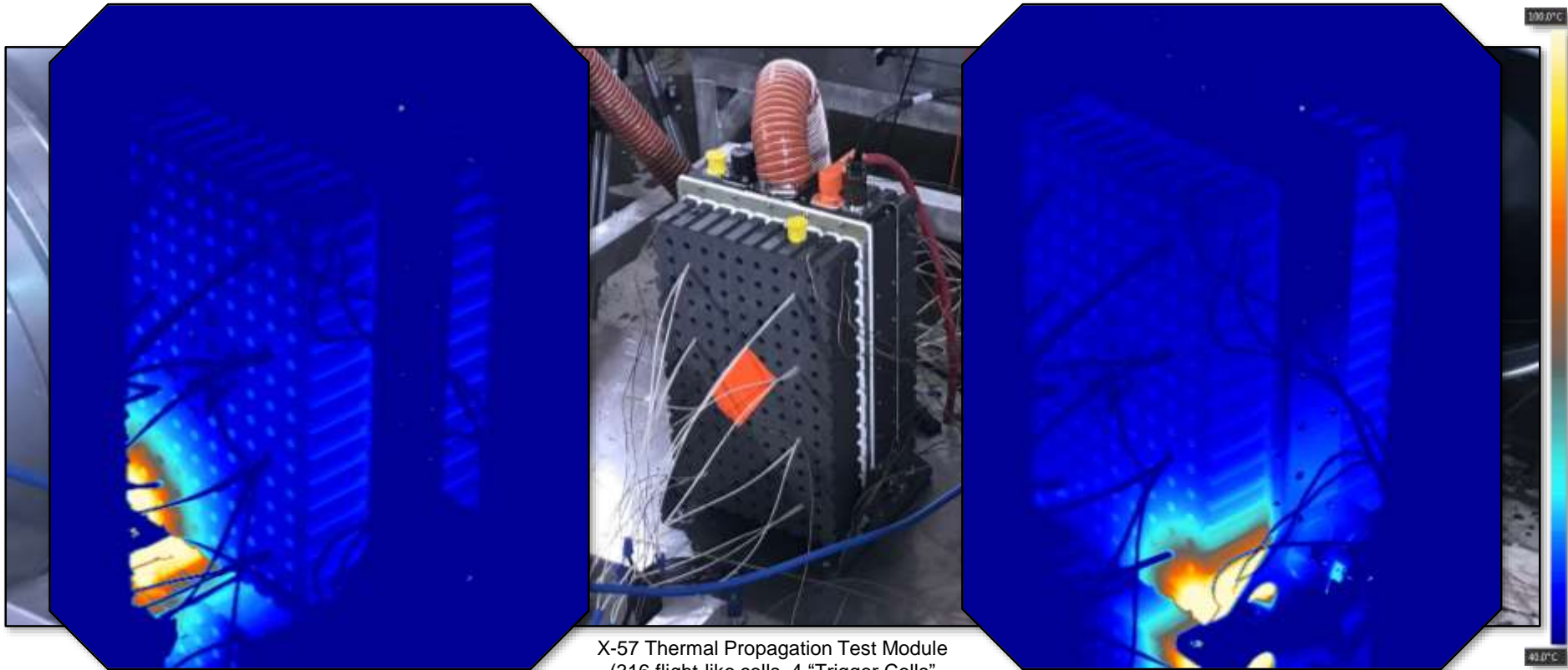
FLIR Video of Trigger Cell #4 Event (8x speed) https://nasa.gov/x57/technical
