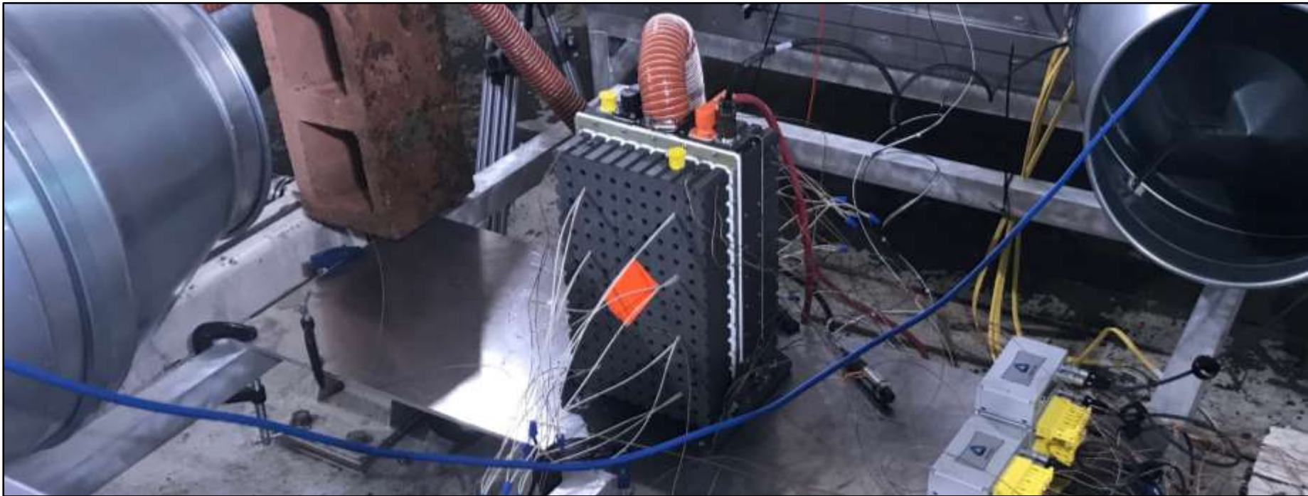
X-57 Thermal Propagation Test Module (316 flight-like cells, 4 "Trigger Cells" with internal shorting devices)
