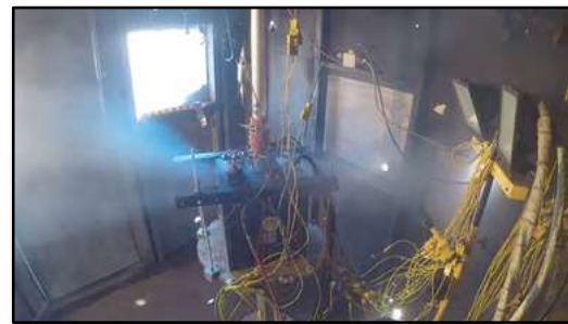
Original battery failed containment propagation test in Dec 2016
