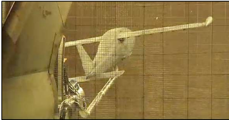
Unpowered Stability and Control Dynamics Test in the 12' Tunnel at LaRC
