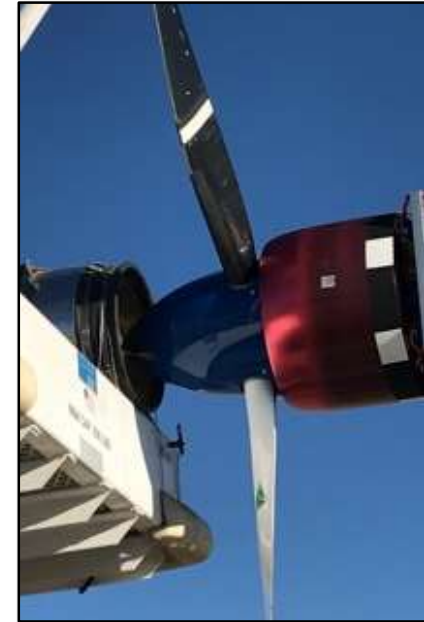
Cruise Motor endurance testing on NASA Airvolt stand at AFRC
