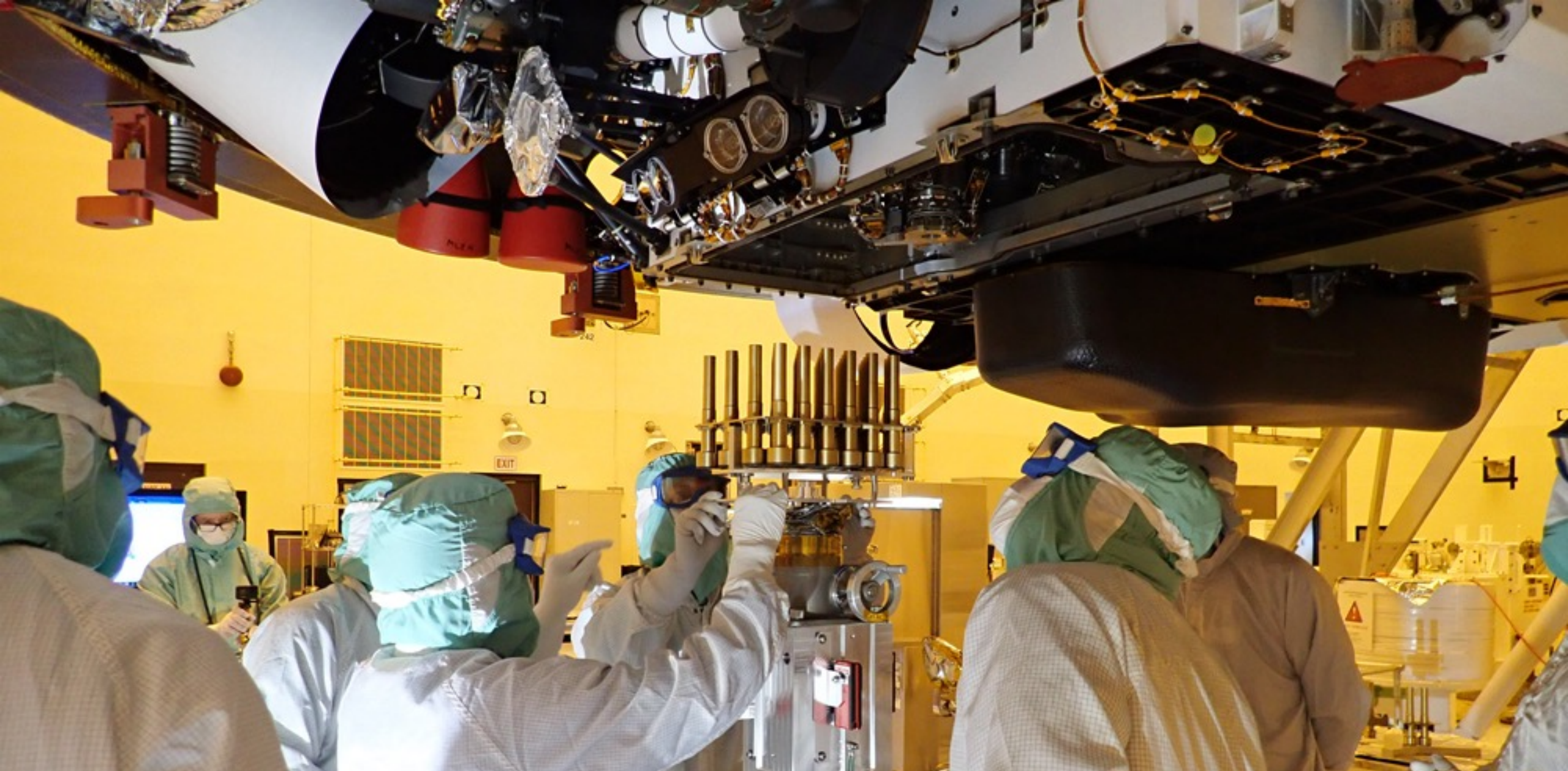
Engineers and technicians working on the Mars 2020 Perseverance team insert 39 sample tubes into the belly of the rover. The rover will carry 43 sample tubes to Mars' Jezero Crater. The image was taken at NASA's Kennedy Space Center in Florida on May 20, 2020.
