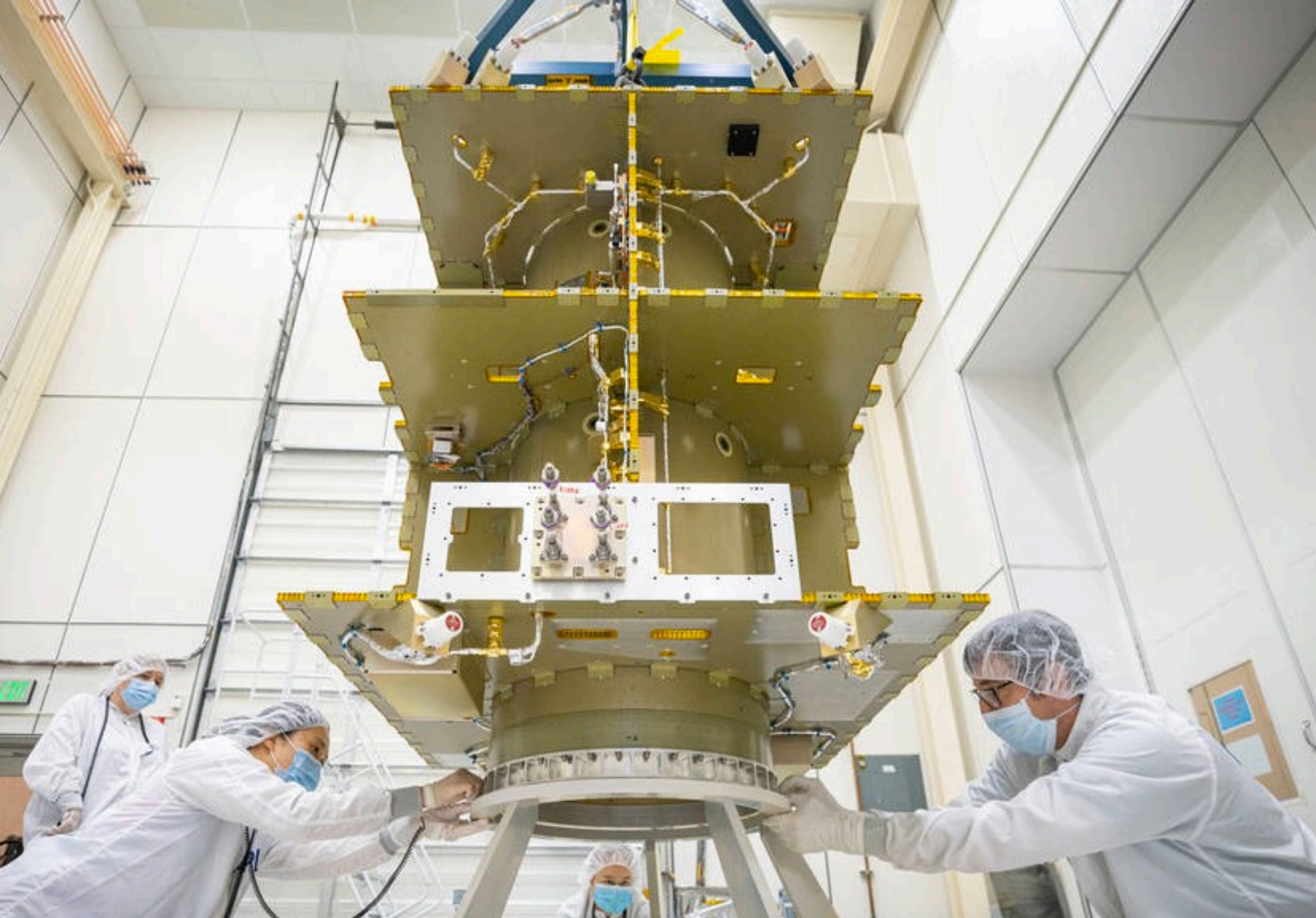
On May 15, the primary structure for NASA's Double Asteroid Redirection Test (DART) spacecraft returned to the Johns Hopkins Applied Physics Laboratory (APL) in Laurel, Maryland equipped with its chemical propulsion system and elements of its electrical propulsion system.
