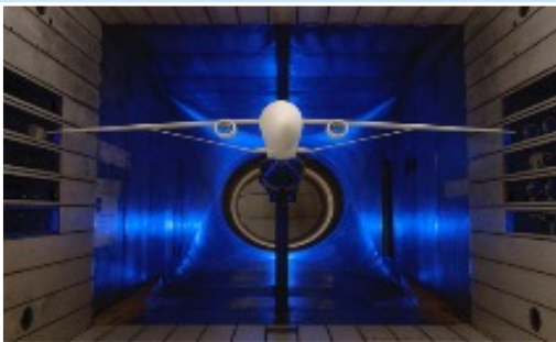
Transonic Truss-Braced Wing 5-10% fuel burn benefit
