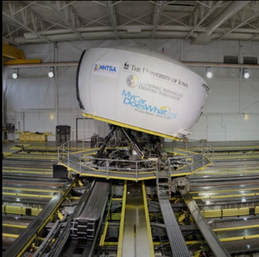
NADS-1 motion base driving simulator
