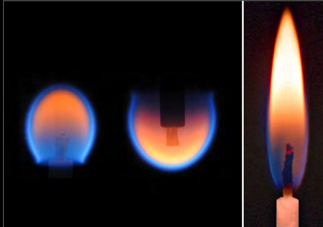
A spherical flame created in space (left), and a candle flame burning on Earth (right)
