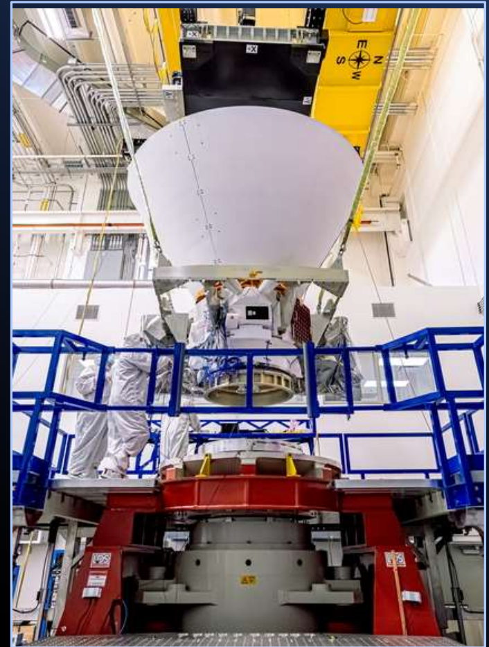
SPHEREx observatory being lifted and installed onto the vibration table, in the Z-axis configuration, at BAE Systems in Boulder CO in early August 2024.
