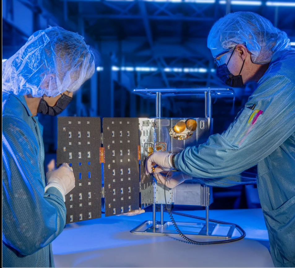
Technicians attach a solar array to one of the Electrojet Zeeman Imaging Explorer (EZIE) CubeSats. Credit: Brooks Freehill, Blue Canyon Technologies
