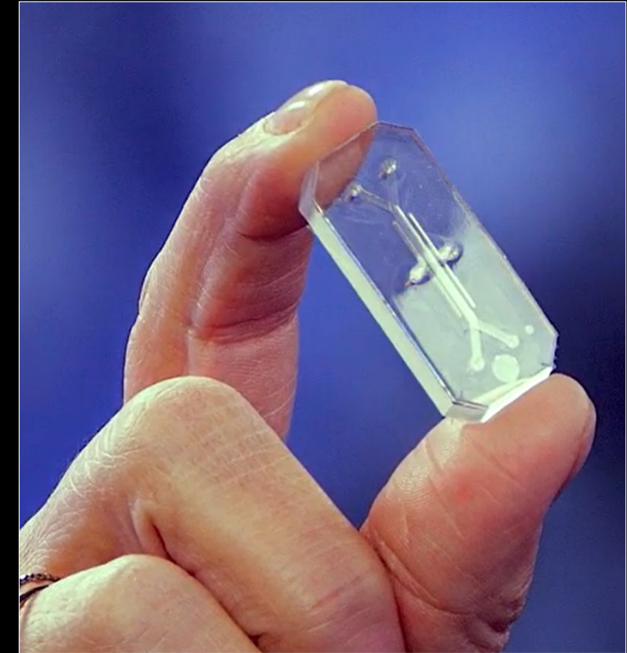
A tissue chip held by Biological and Physical Sciences Division Director Dr. Lisa Carnell. Tissue chips such as this will be used in upcoming space flight research and Artemis missions.
