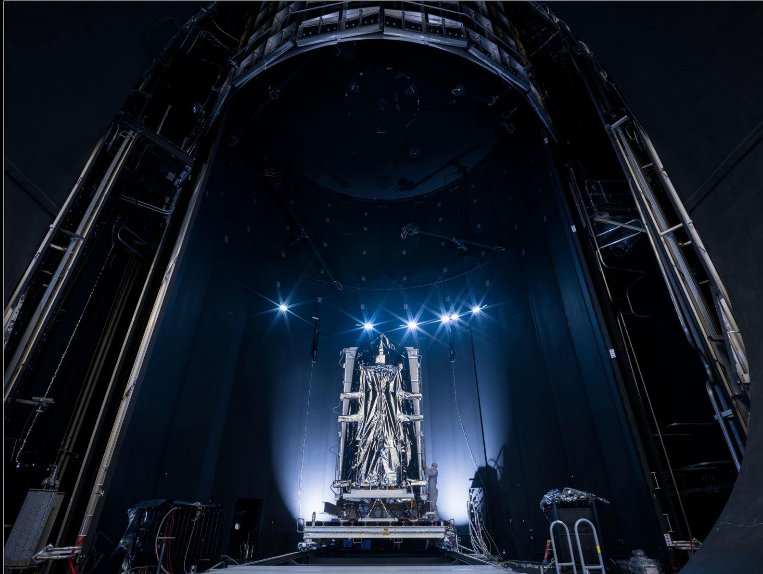
NEO Surveyor Instrument Enclosure Inside Historic Chamber A
