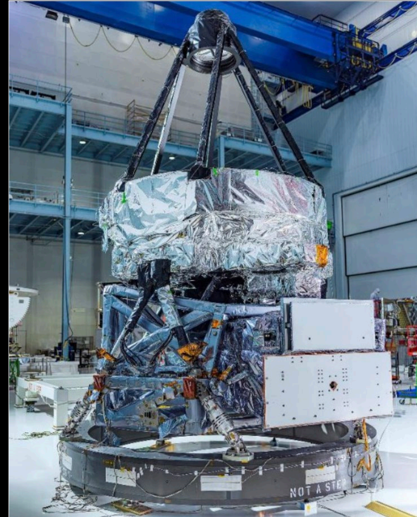
Deployable aperture cover for NASA's Nancy Grace Roman Space Telescope as seen through the outer barrel assembly. Credit: NASA/Chris Gunn
