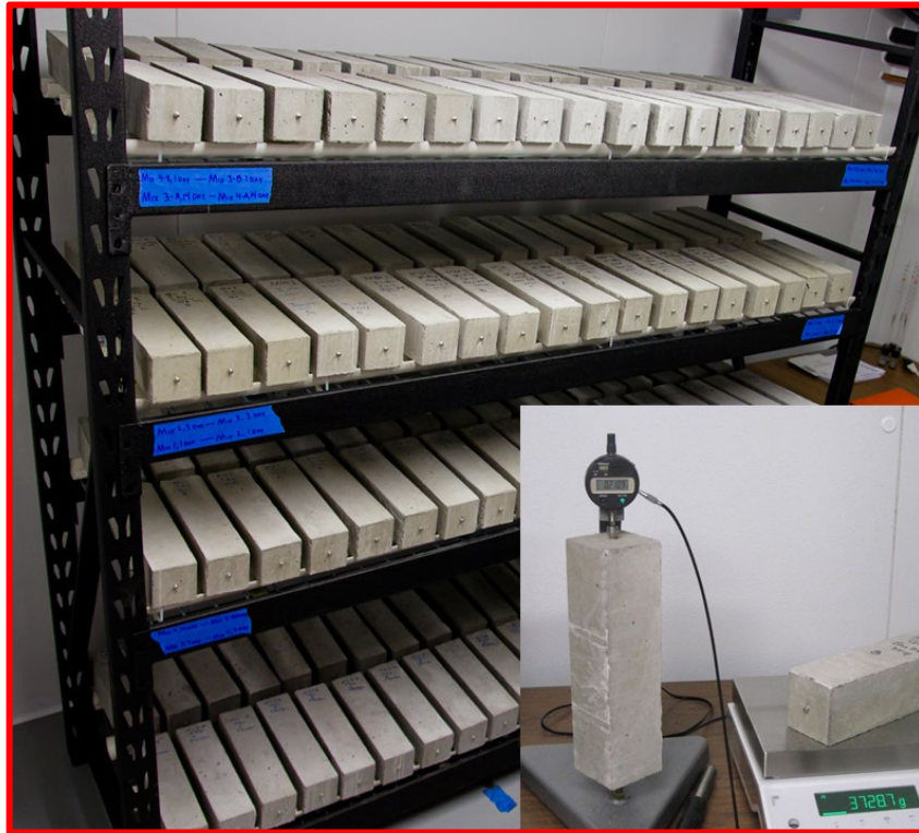
Free Shrinkage Measures total propensity for volume change
