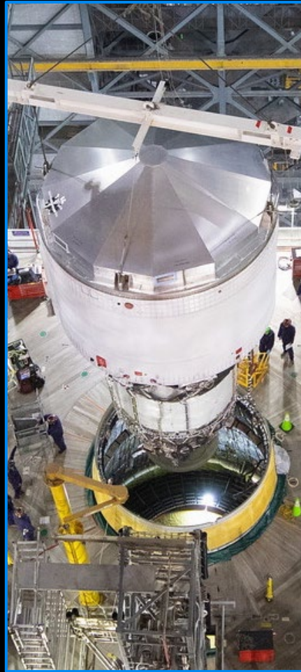
NASA Ground Systems successfully integrated the SLS rocket's upper stage, including the interim cryogenic propulsion stage: May 1, 2025
