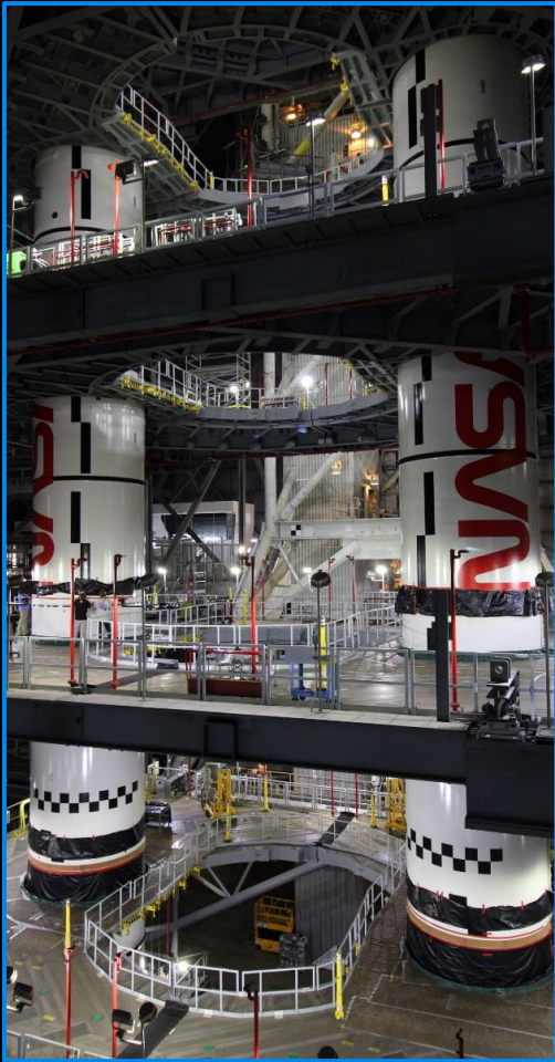
Stacking of the solid rocket boosters completed in High Bay 3 of the Vehicle Assembly Building: February 2025
