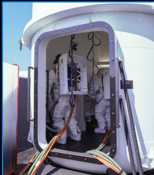
Integrated Artemis III testing: Full-scale airlock, elevator mockup, pressurized suits, HITL: April 2024
