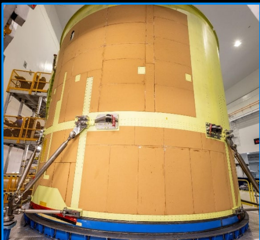
Teams at NASA's Kennedy Space Center installed four "quad pods" around the Artemis III core stage engine section: September 10, 2024
