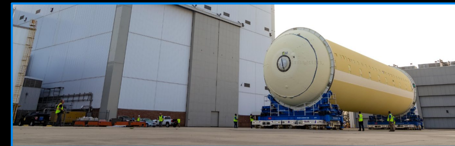
After applying the thermal protection system to the SLS liquid hydrogen tank for Artemis III, teams moved the tank to the final assembly area: May 14, 2025
