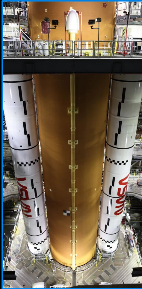
Artemis II Core Stage Integration with solid rocket boosters at NASA Kennedy complete: March 24, 2025
