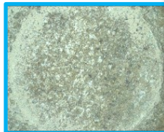
South Arm Abrasion: Cat Arm Reservoir Sample: 2 failed attempts due to 'soft' rock
