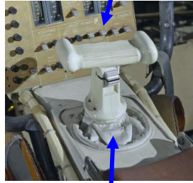
"T" Shaped Hand Controller to Fit Astronaut Glove
