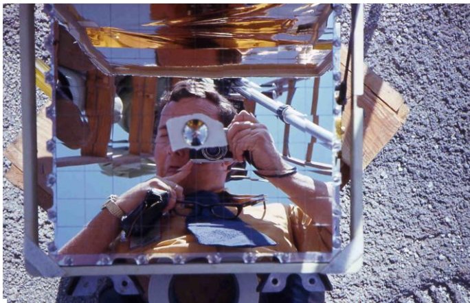
Form Factor Meter Photographed to Validate Model "View Factors" to LM
