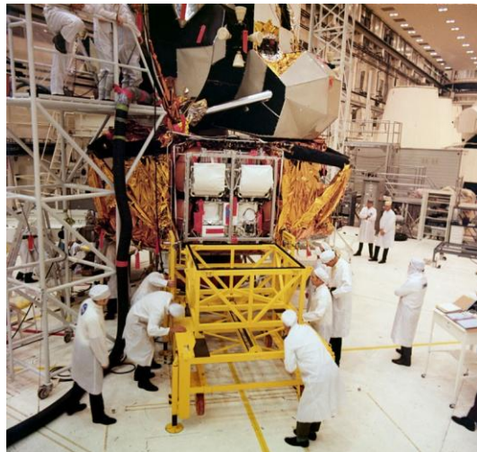
Folded LRV Stowed in Lunar Module with Floor Panels Removed for On-pad Battery Installation
