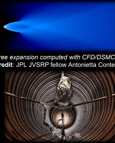
DLR STG-CT test section; thruster pack at center. Image credit: DLR
