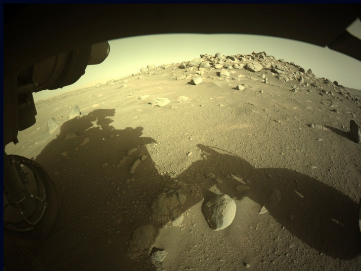
Guarded drive stops rover before rock sol 107 (June 8, 2021)
