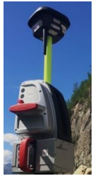
Laser scanners (up to 2.4 km range)
