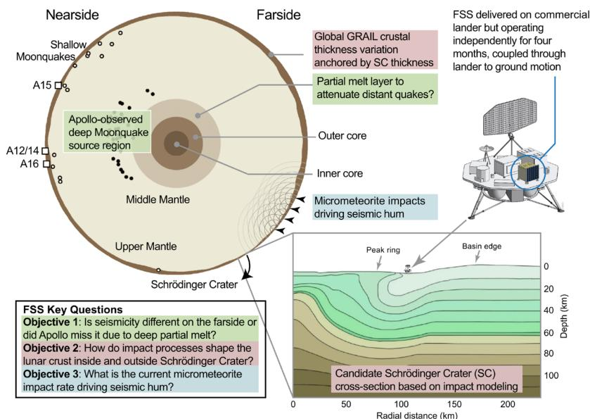
Global cross-section adapted from Wieczorek et al. (2009) and Schrödinger cross-section from Kring et al. (2016)
