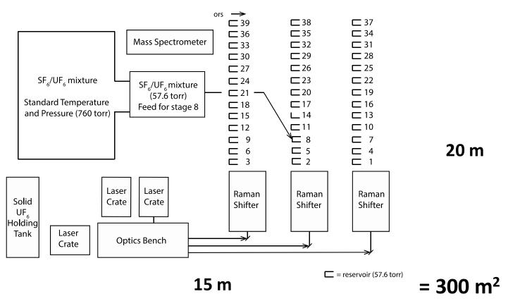
This facility would produce 32.5 kg of HEU per year enriched to 90% in uranium-235. The IAEA defines one significant quantity (SQ) as 25 kg of uranium-235 included in HEU enriched to 20% or greater. For 90% HEU, 1 SQ = 27.8 kg.
