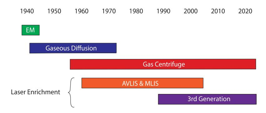
Previous enrichment technologies exploited the difference in mass between U-235 and U-238. Laser Isotope Separation exploits that U-235 and U-238 absorb different wavelengths of light.
