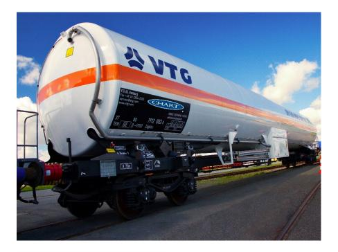
Chart teamed up with VTG, a leading rail logistic company, to develop cryogenic tank cars for the European network
