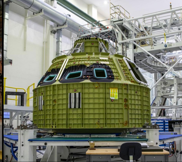
ARTEMIS IV CREW MODULE PRESSURE VESSEL AT KENNEDY SPACE CENTER
