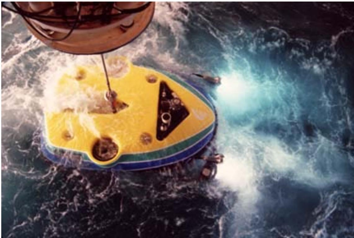
Figure 4. The MBARI ROV *Tiburon*. This vehicle was first launched in 1997 and allows scientists to explore the ocean to depths of 4000 m. Its variable ballasting system and electric motors make it an ideal platform for silently hovering in the midwater to observe animal behavior. Photo by David French ©1997 MBARI.
