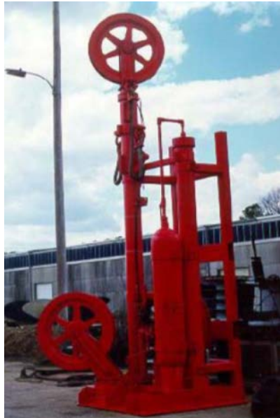
FADOSS 60-Kip Ship Motion Compensator
