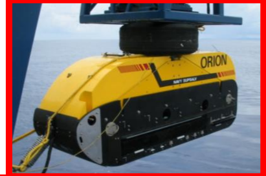
Orion21 Side Scan System Depth - 20,000 ft
