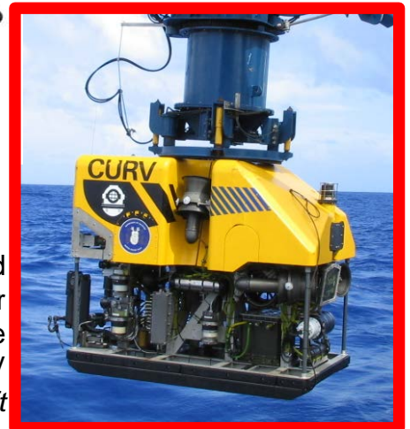
Cable-Controlled Underwater Recovery Vehicle (CURV) 21 ROV Depth - 20,000 ft
