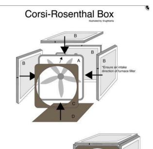
Materials: (A) 1x 20'x20' box fan (B) 4x 20'x20'x1" furmace filters MERV 13'/Filtrete FPR 1900 ('can use MERV 11 if not available) (C) 1 fan shroud made of fan box (D) 1 fan bottom made of fan box - lots of duct tape to seal everything super well
