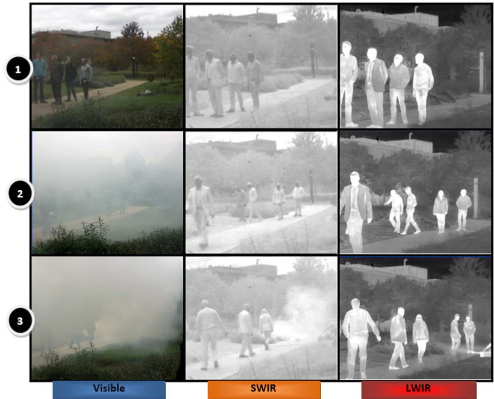
Figure 6 Test at outdoor of visibility in artificial fog
