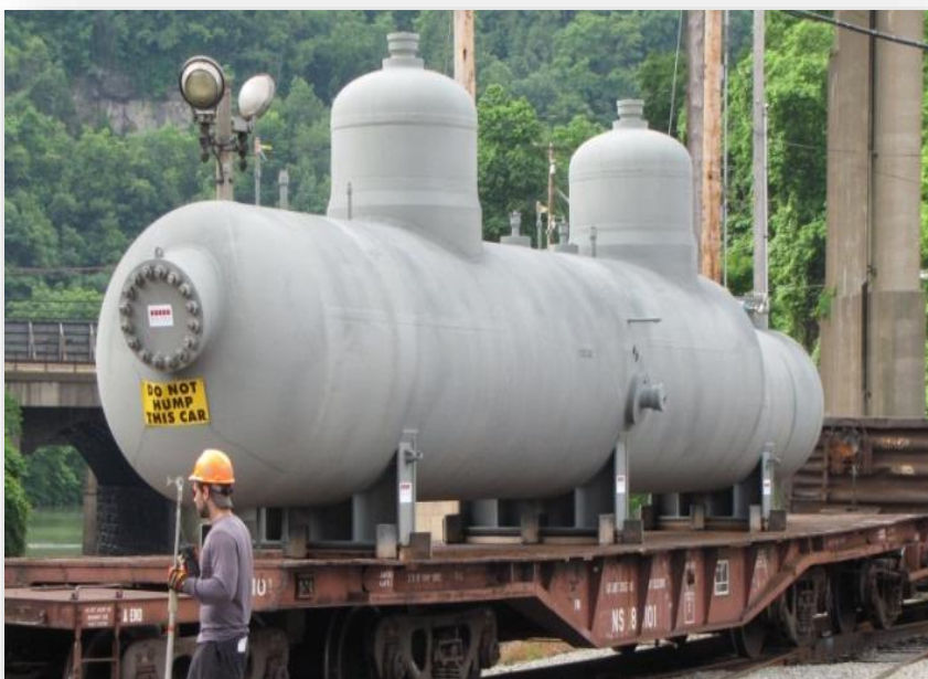
Horizontal Steam Generator
