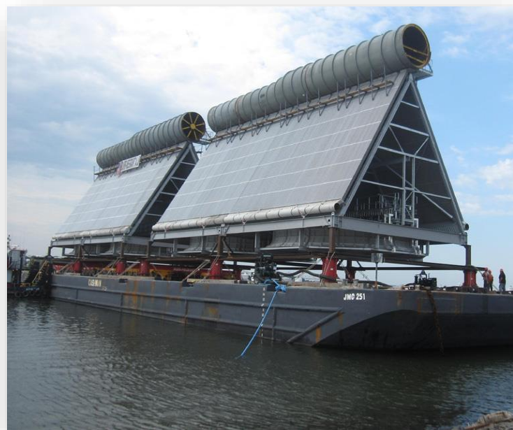
Air Cooled Condensers
