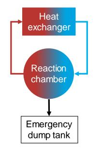
• Intensely radioactive fuel salt pumped at pressure round an engineered system which can never be approached by a human being
