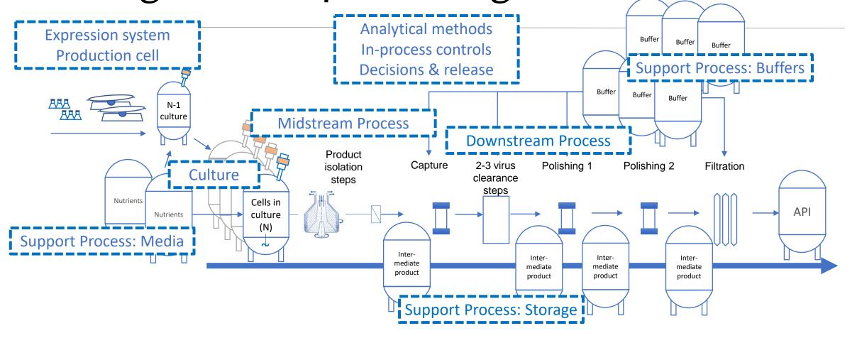
Most process steps can be operated either in batch or continuous mode. Most equipment is available either in single-use or stainless steel.
