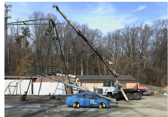
Figure 3. The luminaire support breaks away upon impact.
