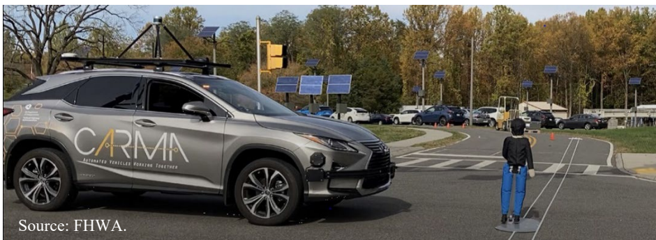
Figure 5. The Human Factors Team testing detection of an articulated child pedestrian dummy.
