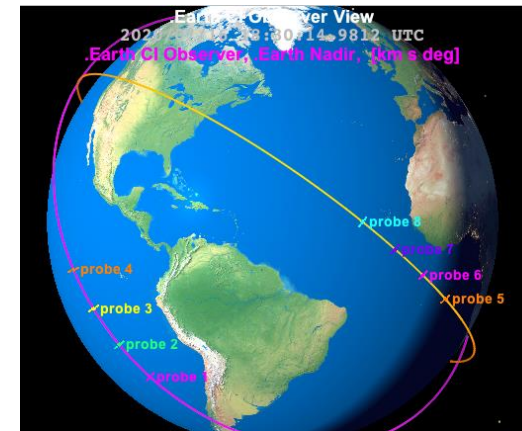
Multiple orbit planes of probe group releases provides horizontal and vertical density resolution.
