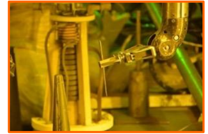
Casting furnace used to fabricate recycled metallic fuels for IRT-1 (JFCS).
