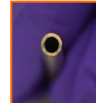
Annular U-10Zr metallic fuel: (1) as-fabricated, and (2) at ~5% burnup.
