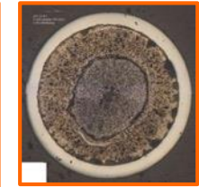
Annular U-10Zr metallic fuel: (1) as-fabricated, and (2) at ~5% burnup.
