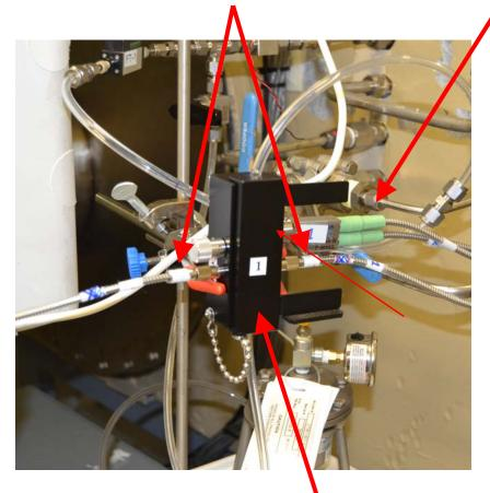
Flow cells installed for real time spectroscopic monitoring of process solutions
