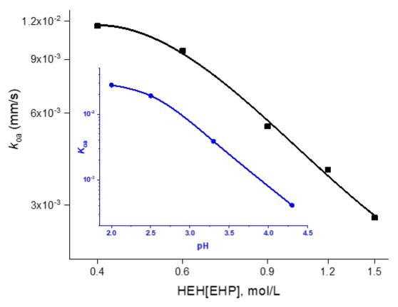
Am backward-extraction rate constant as a function of the HEH[EHP] concentration and the pH of the DTPA buffered solution (inset). Aqueous phase 0.015 mol/L DTPA.0.2 mol/L (H/NH<sub>4</sub>)<sub>3</sub>Citrate, pH 2.0, variable HEH[EHP] conc.; Inset: 0.75 mol/L HEH[EHP]/n-ddn, Aqueous phase: 25 mmol/L DTPA, 0.5 mol/L (H/NH<sub>4</sub>)<sub>3</sub> Citrate, variable pH.
