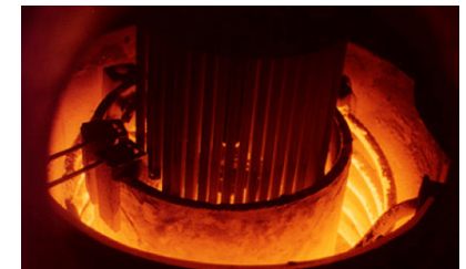
Highly Enriched Uranium pins formed via injection casting
