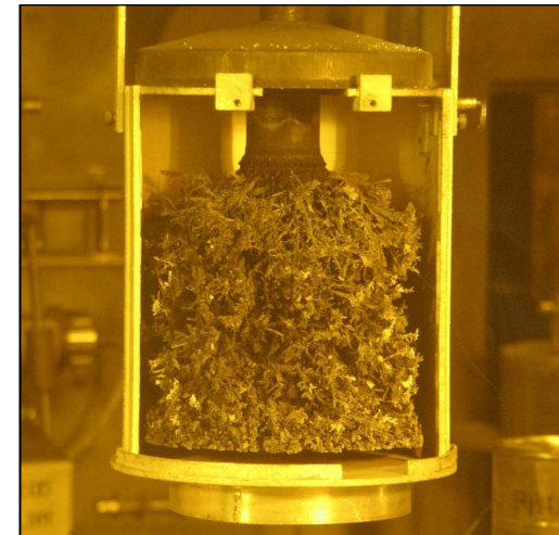
Uranium metal removed from electrorefiner
