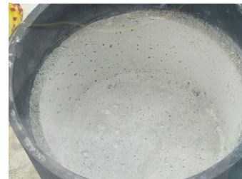
Graphite crucible coated with ZrO 2 , similar to what was used in melt refining
