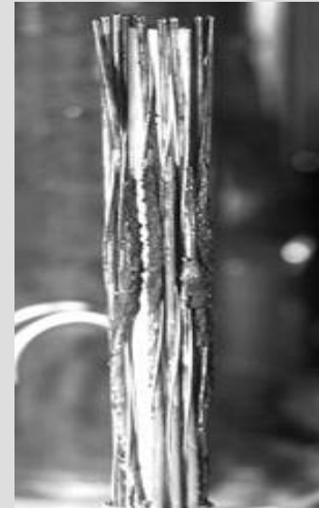
Failed elements recovered from wet storage
