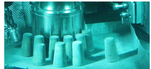
Recovered uranium metal in regulus form
