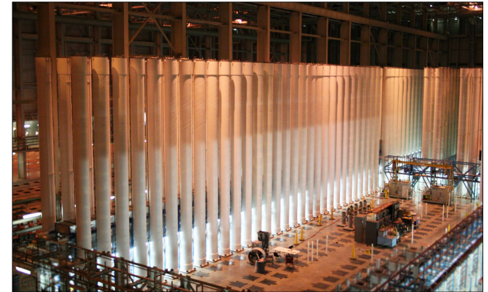
Large Centrifuges for Uranium Enrichment at the American Centrifuge Plant
