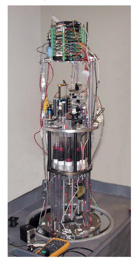
Figure 7. The MBARI Environmental Sample Processor (ESP). This device is designed to conduct autonomous, preprogrammed deployed in the ocean environment. Samples can also be preserved for later analysis in the laboratory after the filters are chemical processing (such as DNA probe arrays) on material collected, filtered, and concentrated from seawater while recovered. Two-way communication with the shore is provided by radio modem. Photo by Todd Walsh ©2001 MBARI.
