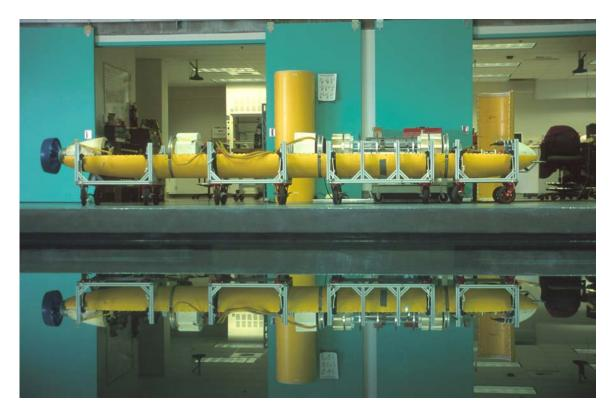
Figure 6. The MBARI AUV *Dorado*. The vehicle can be configured in lengths from 2.2 m (no midsections) to 5.6 m (two midsections). The vehicle minimizes the use of pressure housings by putting most systems in smaller, lighter, oil-filled enclosures. Its depth rating is 4500 - 6000 m, depending on the payload. The vehicle is steered by a novel articulated tail cone and propelled by a ducted propeller, resulting in more robust, efficient operation. Photo by Todd Walsh ©2001 MBARI.
