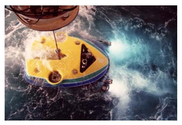
Figure 4. The MBARI ROV *Tiburon*. This vehicle was first launched in 1997 and allows scientists to explore the ocean to depths of 4000 m. Its variable ballasting system and electric motors make it an ideal platform for silently hovering in the midwater to observe animal behavior. Photo by David French ©1997 MBARI.
