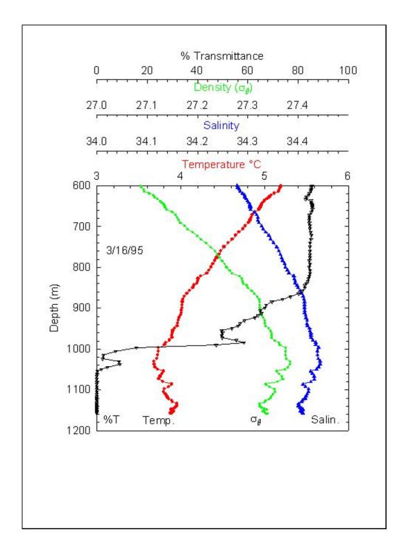
Figure 10. Record from MBARI's ROV *Ventana* as it descended into Monterey Canyon on March 16, 1995. The physical parameters show a near-bottom inversion as the ROV entered what appears to be a hyperpycnal flow from the Salinas River.
