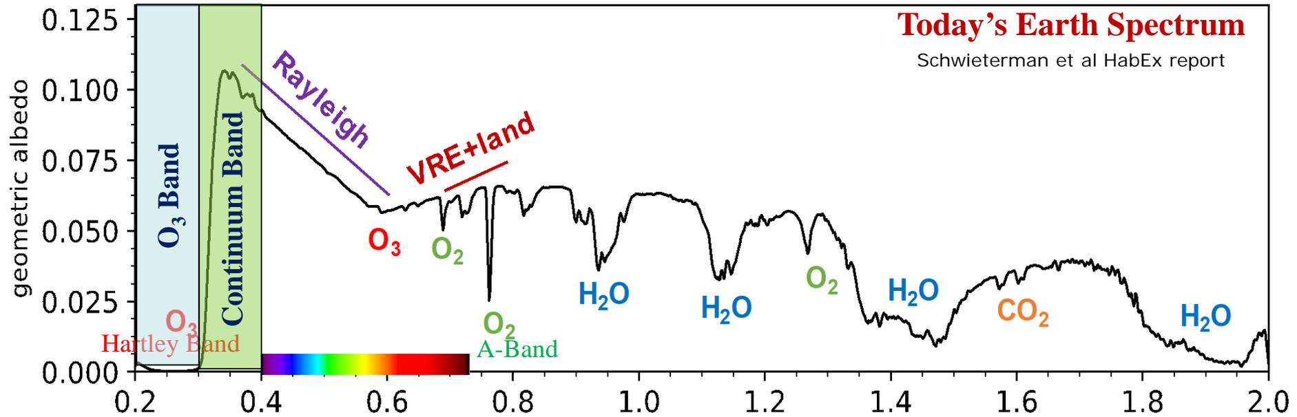
*O<sub>2</sub> A-Band detection requires SNR of 20 per Feng et al 2018.*
