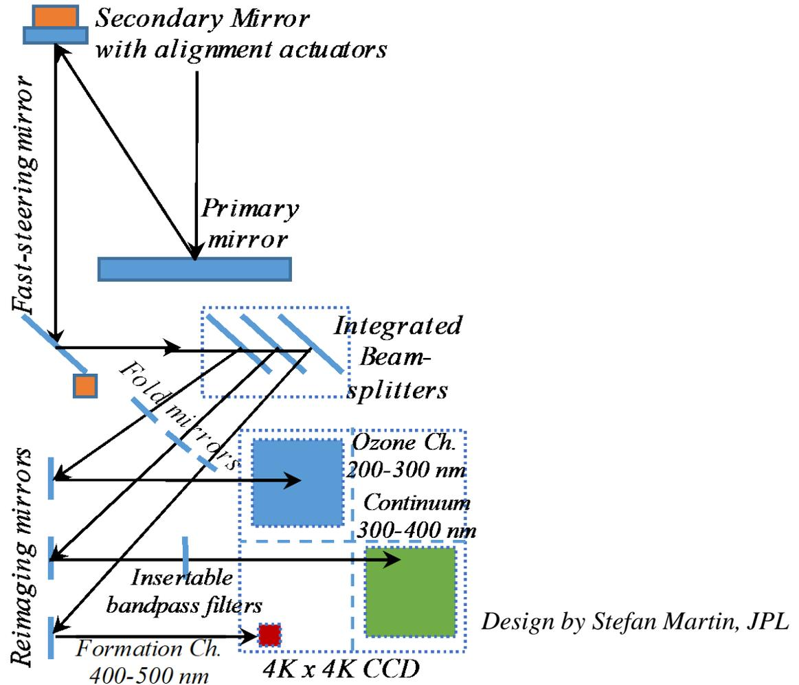
*A simple 2-channel photometer can detect the presence of Ozone.
