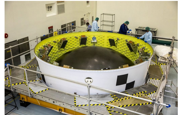
All 10 secondary payloads have been installed in the Space Launch System (SLS) rocket's Orion stage adapter.
