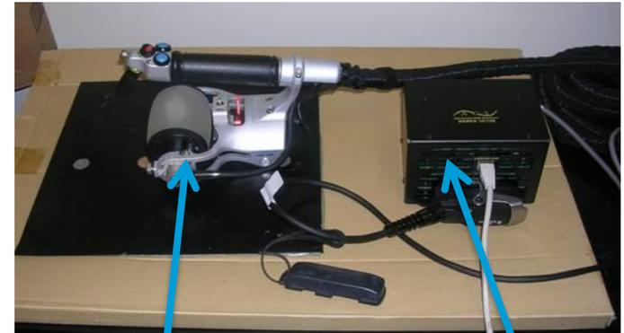
Phased Array in a Roller Housing
